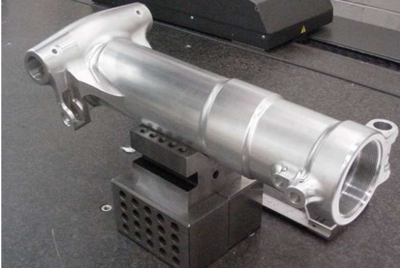
Newly manufactured wing landing gear main strut. http://merrillaviation.com/capabilities/aviation-capabilities/aviation-landing-gear
