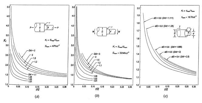
Fig 9.3 Stress concentrations factors for a stepped shaft (a)Tension, (b)Bending, (c)Torsion
