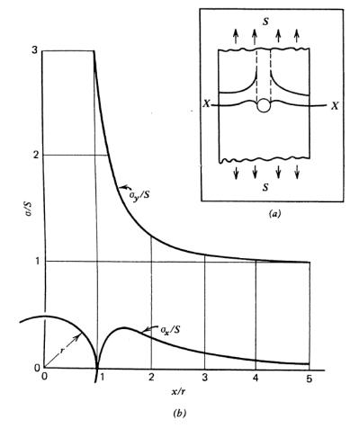
Fig. 9.2 Stress distribution along the section X-X near a hole in a wide sheet Values of  $\sigma_y/S$  and  $\sigma_x/S$  are plotted versus x/r in Fig. 9.2. We see that  $\sigma_y/S$ decreases quite rapidly as the distance from the edge of the hole is increased.  $K_t$  at the
