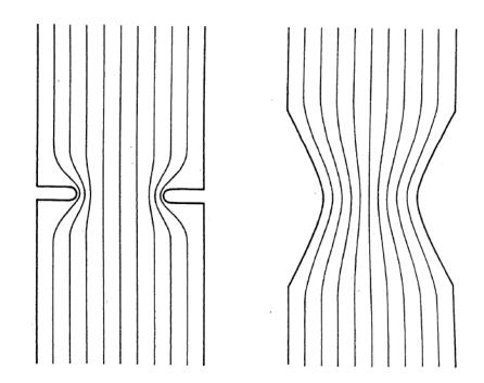
Fig. 9.5 The crowding and bending of flow lines near obstructions helps to visualize the concentration of stresses and strains near notches. The large section and the small section are the same in both cases, but the transitions are different
