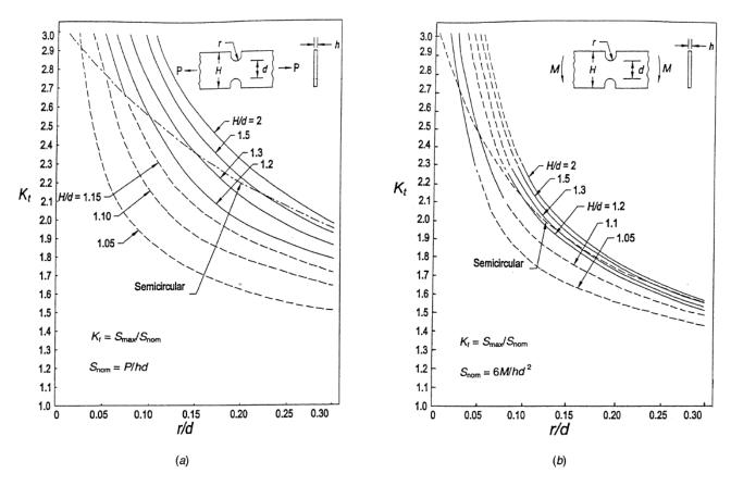
Fig 9.4 Stress concentrations factors for a flat bar with opposite U-shaped notches (a)Tension, (b)Bending
