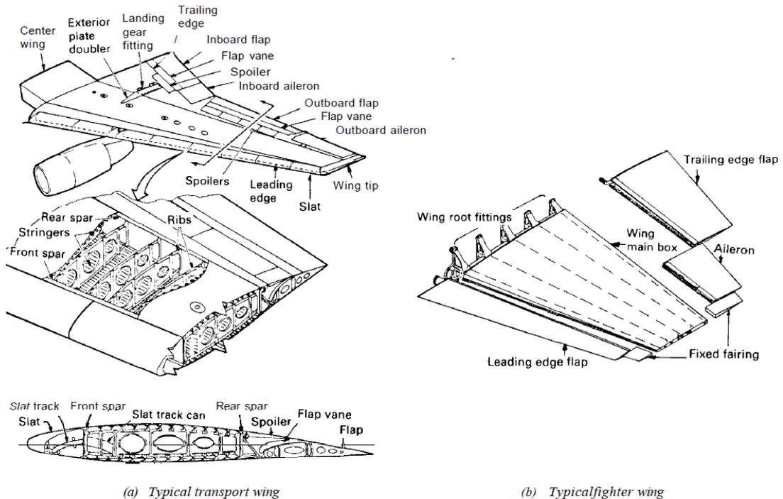
Fig. Typical transport and fighter wings
