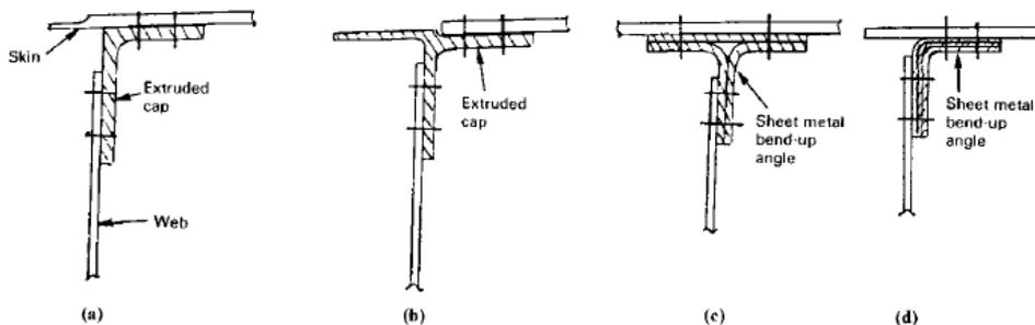
Fig. 8.4.1 Typical spar cap sections.
