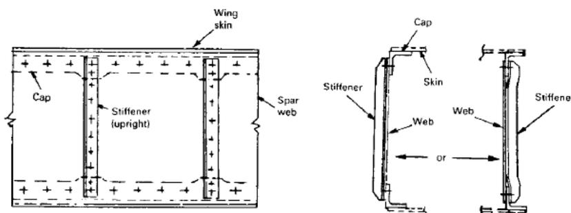
Fig. 8.4.2 Typical spar construction.
