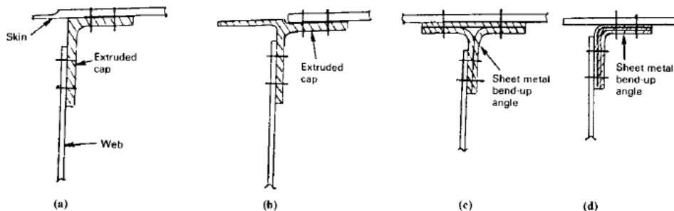
Fig. 8.4.1 Typical spar cap sections.
