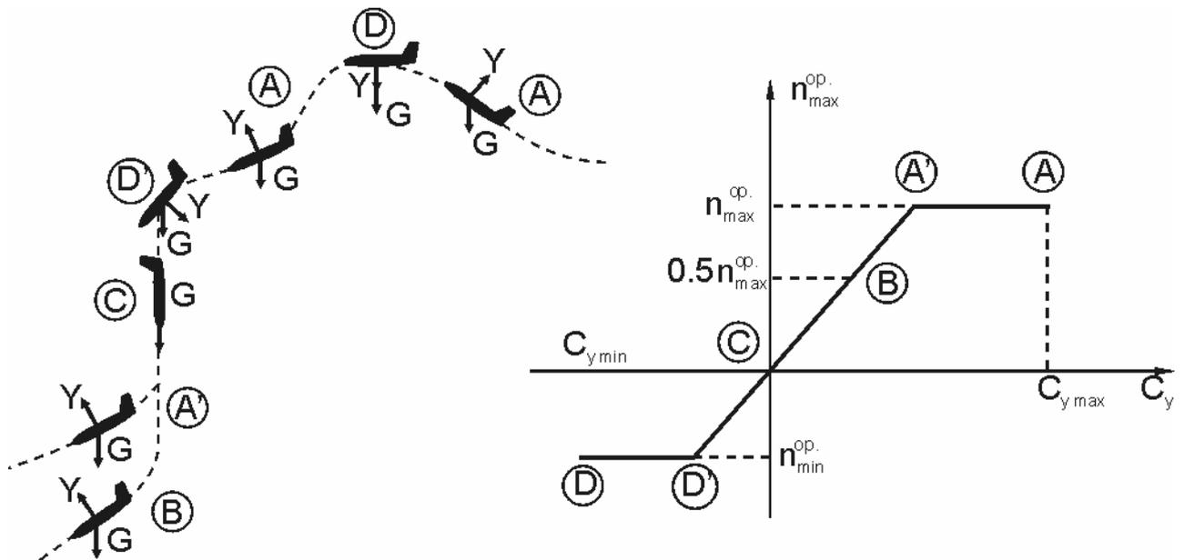
Fig. 3.1. Design Cases of Airplane Wing Loading
