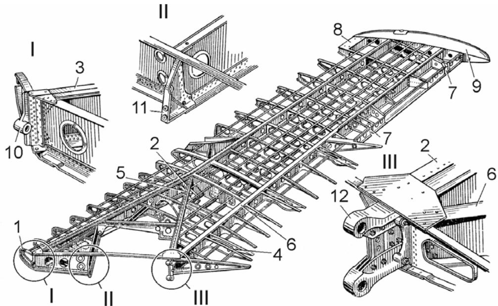
1 – rib; 2 – inner brace; 3 – spar; 4 – flap rails; 5 – MLG attachment fitting;
