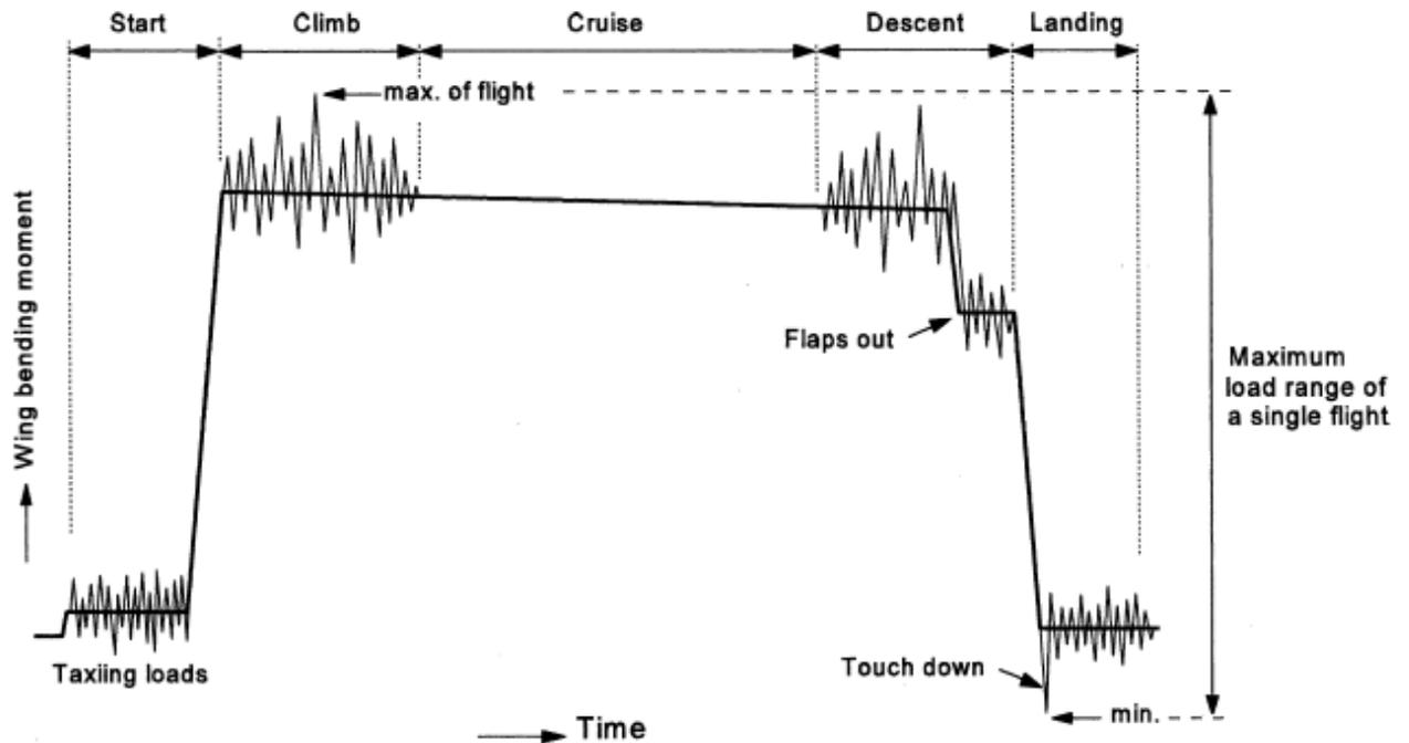
Fig. Slow load variation of the wing bending moment during a single flight, with fast superimposed turbulence loads and ground loads.
