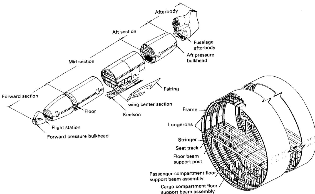
In addition to stabilizing the external skin, stringers also carry axial loads induced by the bending moment. Frames primarily serve to maintain the shape of
