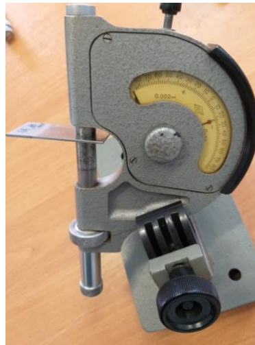
Fig. 5. Measuring the thickness of the sample-plate
