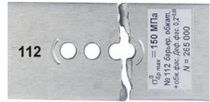
Fig. 6.21 – Fatigue Failure Nature of Strips with Three Holes
