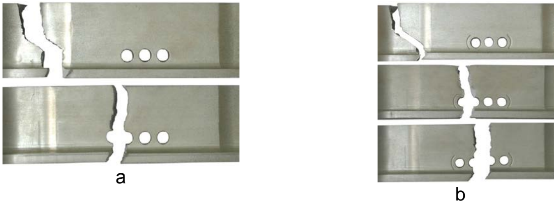
Fig. 6.24 – Structural Stringer-Like Test-Pieces with Functional Holes. Fatigue Failure Area and Nature
