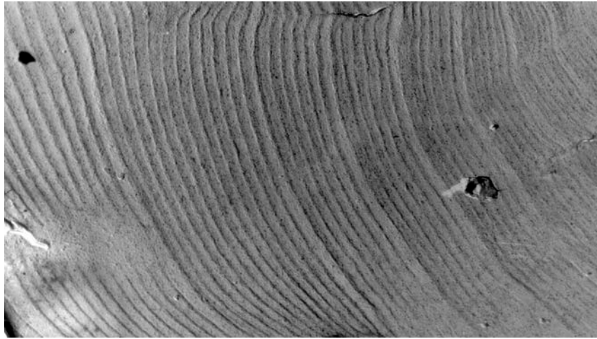
Fig. 8.5 – Test-Piece Fatigue Crack Surface View in Units Replacement Area under Testing in Accordance with Program, Fig. 8.4 (electronic fractogram X6000)
